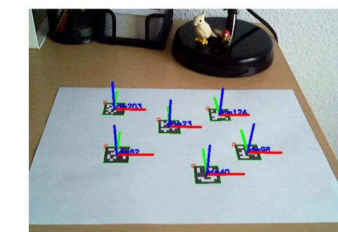
Each Aruco tag is composed of black and white squares that gives each tag a unique ID and a specific orientation. By analyzing the pixel length of each grid square and then referencing a known library of tag ID's and dimensions, a program can calculate the camera's distance and orientation relative to a specific tag [1,2].
