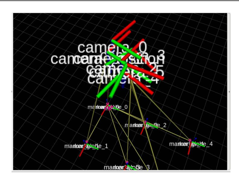
A coordinate axis is superimposed onto each detected marker, and the camera's position is estimated relative to each marker.
